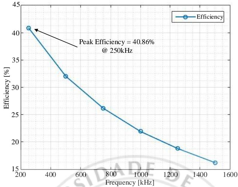
Figure 24 The efficiency of the MEMS Drivers
