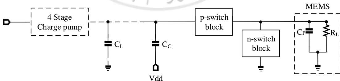
Figure 20 The schematic of the circuit with charge sharing compensation capacitor  $C_c$
