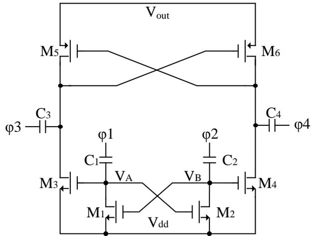
Figure 7 The proposed architecture of the charge pump
